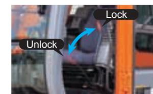
Pilot-control shut-off lever
